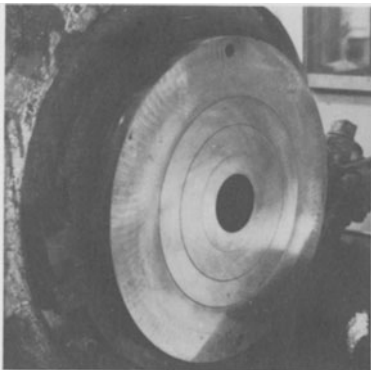
Figure 3 View of the "die-side" of the container and its four press-fitted rings.
